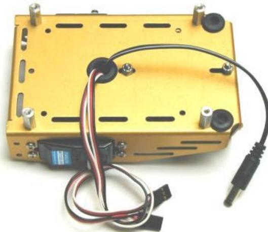
(b) wires pulled through.
