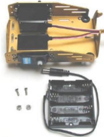
Figure 1.9: Battery pack and mounting hardware.
