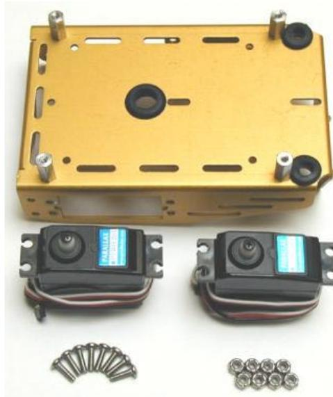
Figure 1.7: Servos and mounting hardware.
