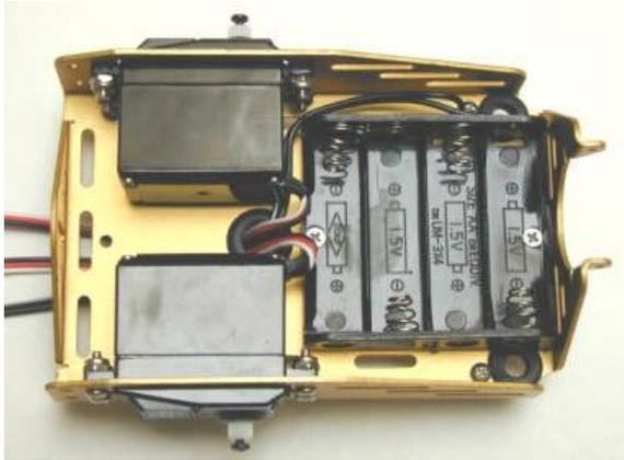
Figure 1.10: (a) Battery pack installed
